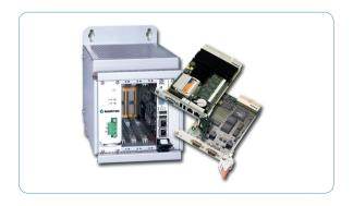
Eickhoff shearer loaders use modular CompactPCI® hardware from Kontron and the CoDeSys Soft PLC together with Profibus and CANopen in a single-system solution. The bundle can also be purchased as a preconfigured, application-ready platform for any control application. In addition to the timesaving hardware/software integration, customers benefit from the ability to customize the system with in-house CPU cards and I/O assemblies.
