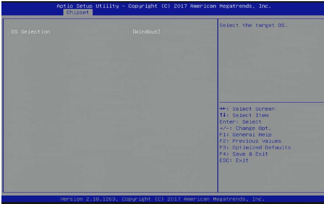
Figure 11: Chipset > South Bridge Menu Initial Screen
