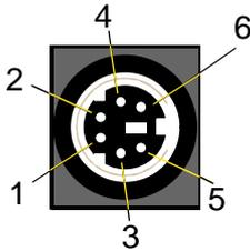
**Figure 2-5: Keyboard/Mouse Connector**
