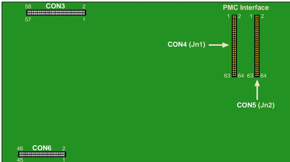
Figure B-2: PMC Module Layout, Version without CPCI Connectors (Rear View)
