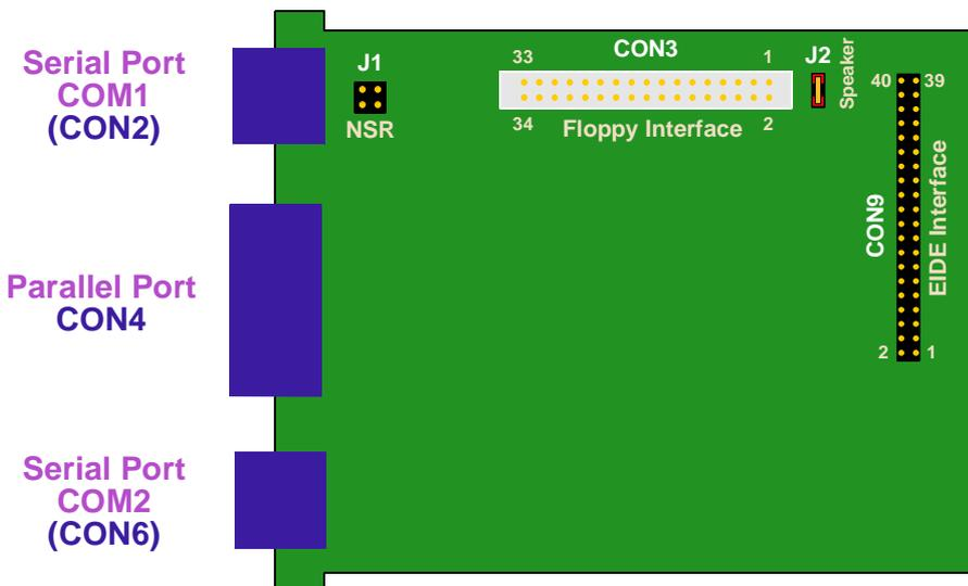
Figure A-2: I/O Module Layout, Standard Version (Reverse Side)
