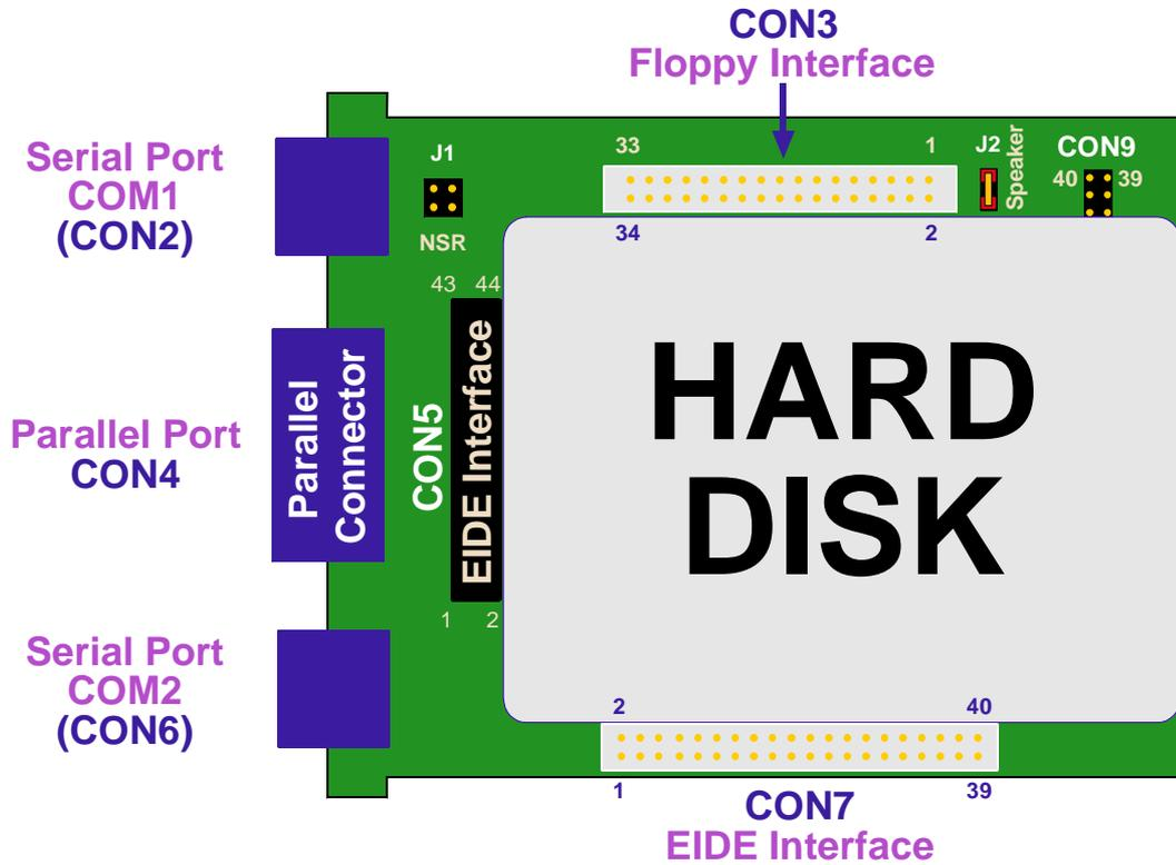
Figure C-4: IDE2 Module Layout, HardDisk Version (Reverse Side)
