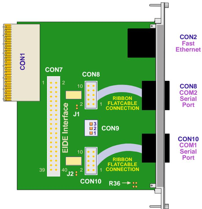
Figure D-3: CP-RIO3-01 Module Layout, 8HP Version
