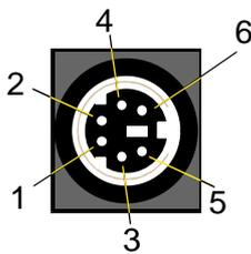
**Figure D-4: Keyboard/Mouse Connector**
