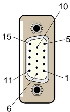
**Figure 2-7: D-sub VGA Connector**
