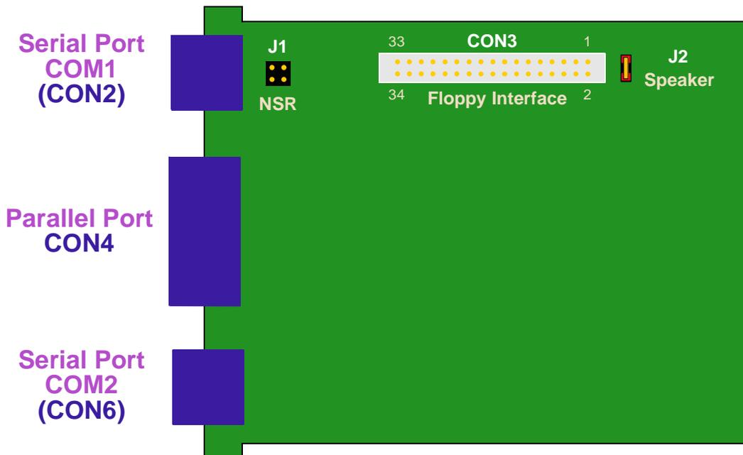
Figure C-2: IDE2 Module Layout, Standard Version (Reverse Side)
