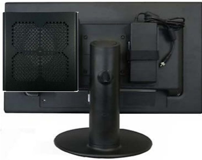
Figure 31: Installed VESA 100 Mount Assembly – non VESA Stand Monitor
