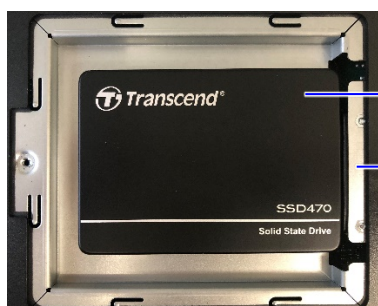
Figure 11: External Drive Bay with 2.5" SSD Drive
