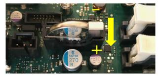
Remove the battery using your fingers or a suitable (non-metal) tool to pull the lithium battery out of the battery holder.
