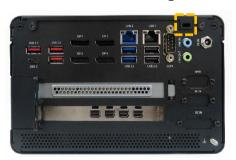
4. Remove the two top cover screws on the rear panel and retain the screws for later use.
