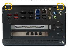
5. Lift the top cover a few centimeters at the rear of the chassis and pull the top cover gently away from the front panel to release the top cover from the front-panel-holding-brackets.
