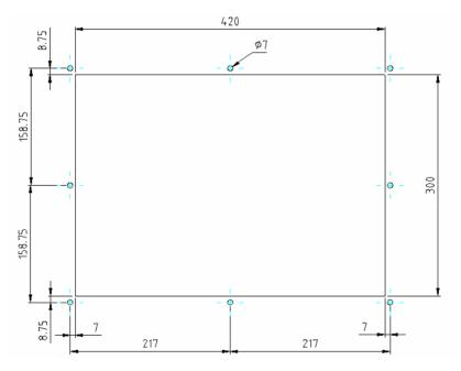
Fig. 6: Hole pattern for the KFM15\_e, Panel mounting (all values in mm)
