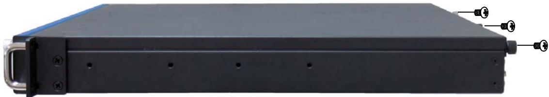
Fig. 15: Loosening the three fastening screws on the rear side of the KISS 1U Short system
