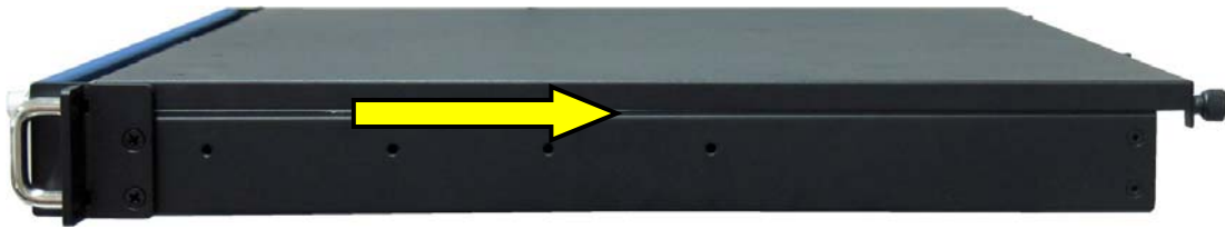
Fig. 16: Sliding the cover back will pull out the cover fixing brackets from the retaining brackets of the chassis
