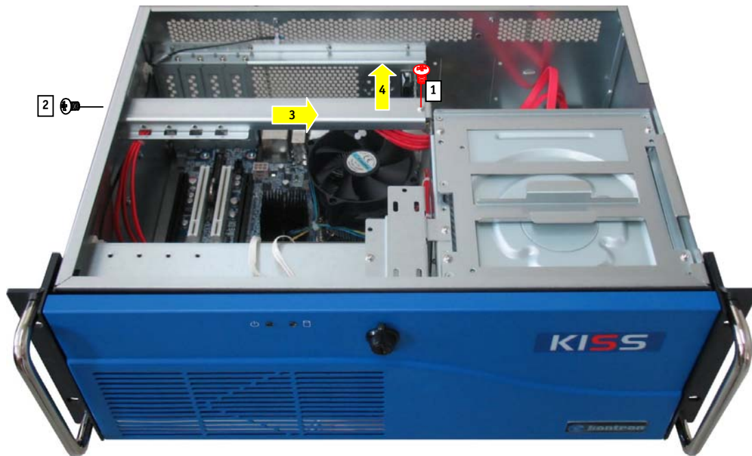
Fig. 29: Opened KISS 4U Short V2 platform - removing the card hold down brackets
