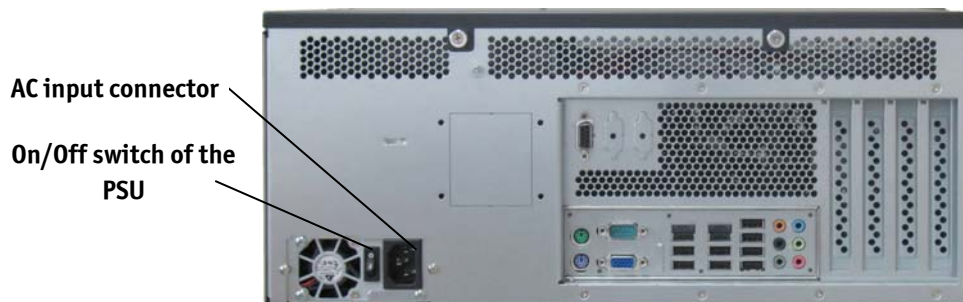
Fig. 30: KISS 4U Short V2, rear side without PE marked grounding stud
