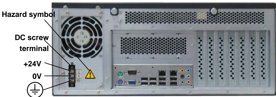
Fig. 23: KISS 4U-System (example) - DC Connection (permanently connected)
