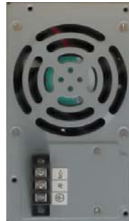
Fig. 14c: Detail - +24V DC PSU
