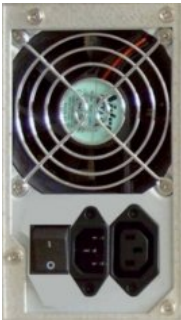
Fig. 14: Detail - Wide Range PSU 300W (AC)
