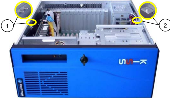
Fig. 21: Bolts and fastening point for the card hold-down bracket
