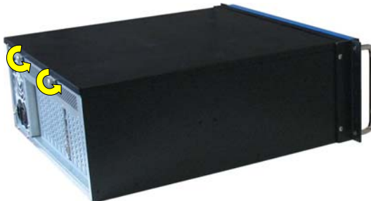
Fig. 17: Loosen the captive knurled screws
