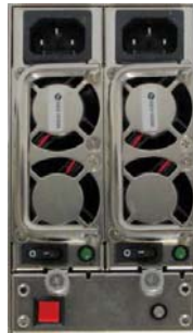
Fig. 14b: Detail - redundant Wide Range PSU (AC)
