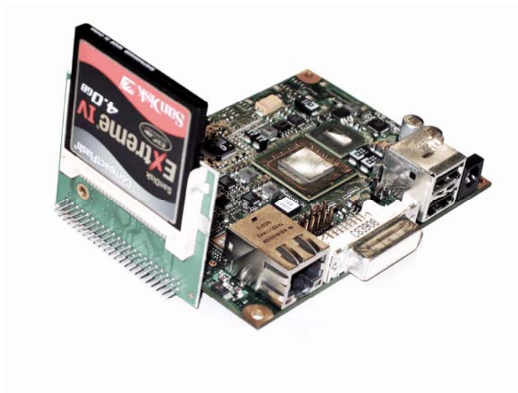
KONTRON CF card adapter (CF-CARD-adapt-MOPS, part number 40404)
