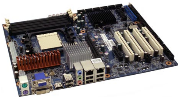
Figure 1: The Kontron KT780/ATX basic motherboard with integrated ATI Radeon HD 3200 graphics
